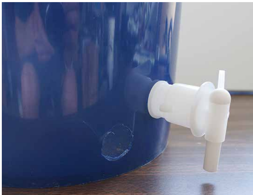
Fig. 5.5: Spigot installed properly. The bucket can sit flat. Note the improperly placed hole.
