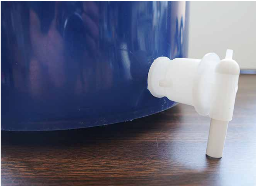
Fig. 5.4: Spigot installed too low. The bucket cannot sit flat.
