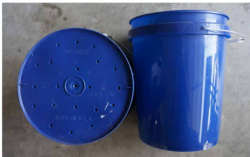
Fig. 5.1-3: Holes drilled into the bottom of the inside bucket.
