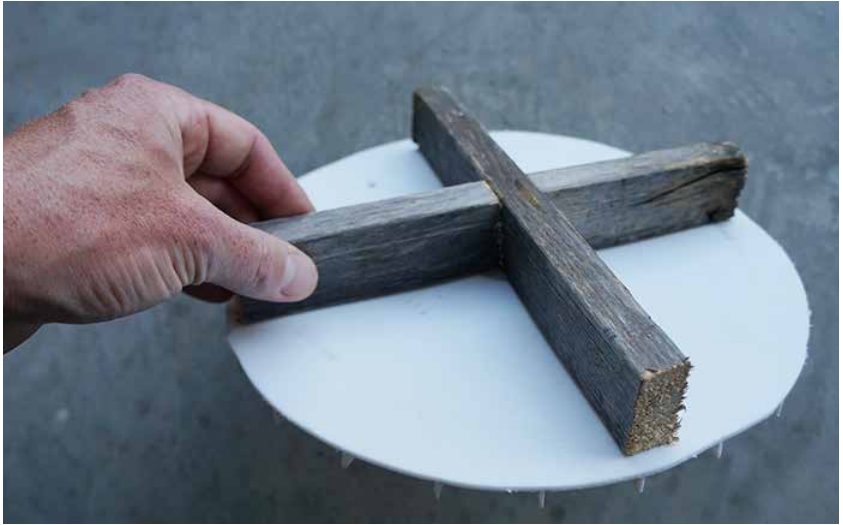
Fig. A.3: Finished pressure plate. An old bucket lid with wood supports.
