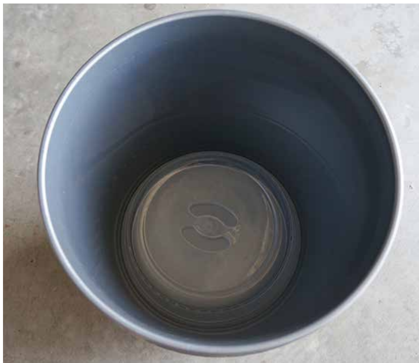
Fig. 5.7: Microwave splatter guard used in the bucket as the divider screen.
