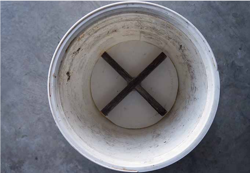
Fig. A.2: Pressure plate inside a five-gallon bucket.
