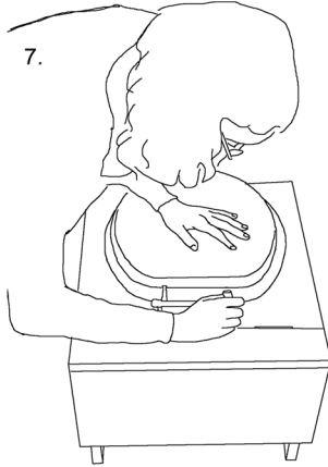
7. Mark holes for toilet seat attachment.
