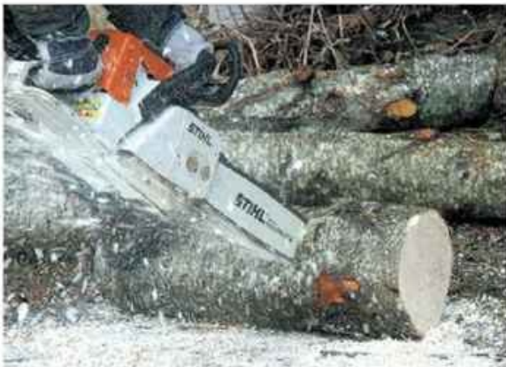
Notching the logs
