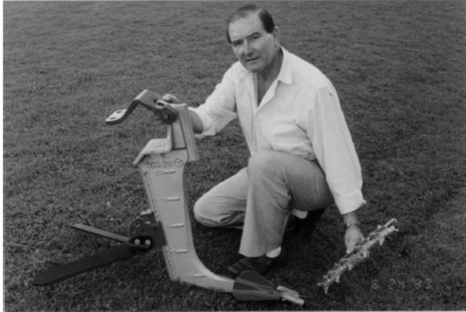
Plate 54 Allan Yeomans shows three of his patents. Rigid, simple shear pin system uses inexpensive round steel bar. New “Leap Frog” digging points fit behind used ones, which means no throw away metal. Self locking track down the back of the tyne enables quick tool changes. Photo shows weed knives attached.
