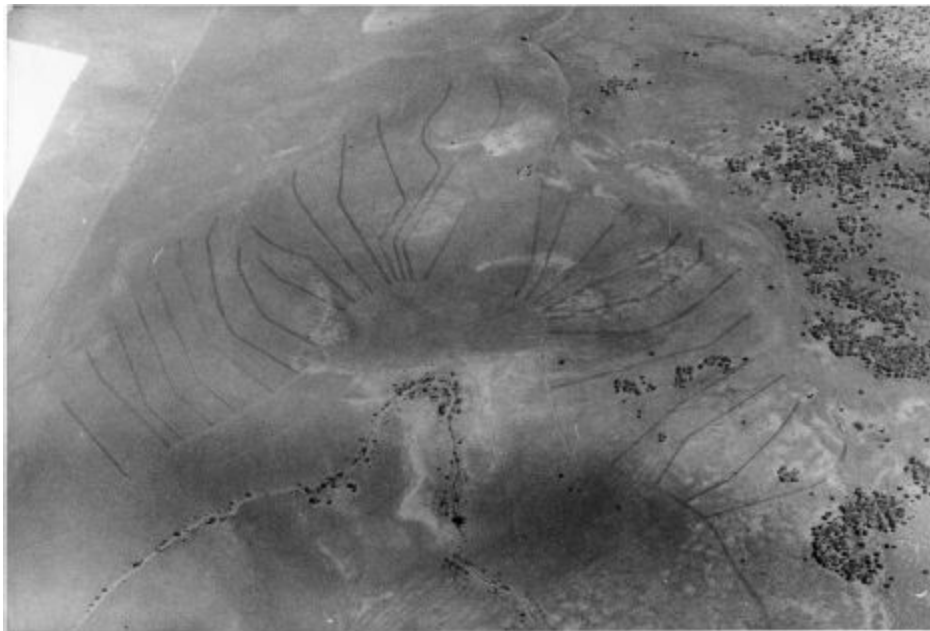
Plate 44 Aerial view of a flood flow layout near Hughenden Qld. It is more practical to split a widening bay by starting a new steering bank well down from the channel rather than have long narrow bays as shown here. The starting point for that bank is selected to appropriately divide the flow of water.
