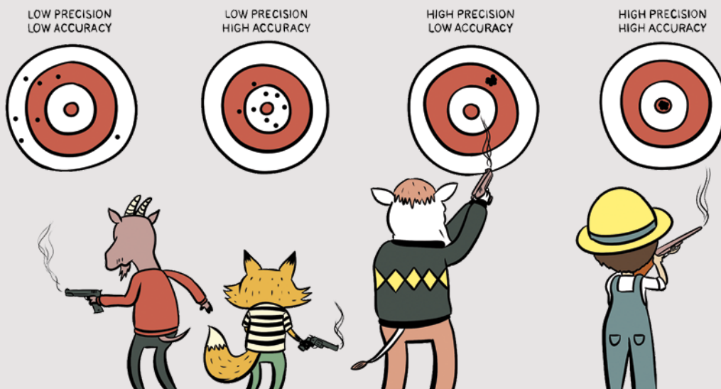
FIGURE 2.7. Precision versus accuracy.
