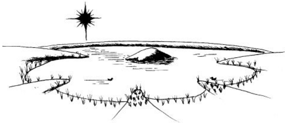
Figure 2.15 Change the shape of a dam to increase the edge and, therefore, the production of the system.
