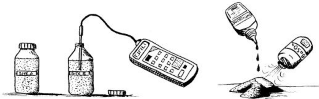
Figure 5.7 Electronic meters are more accurate, but more expensive, than powder test kits.
