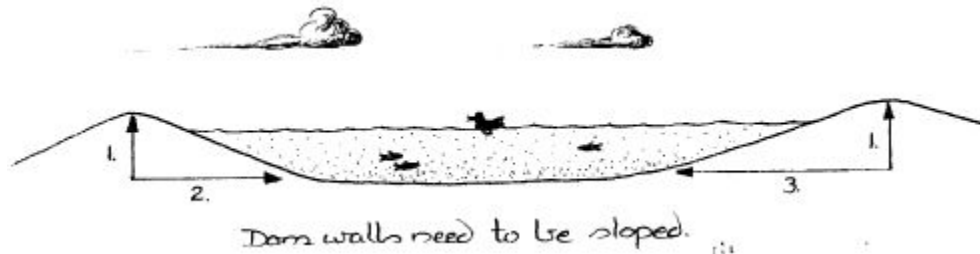
Figure 9.12 The slope of dam walls should be such that they don't cave in. Slopes of 1:2 (27°) or 1:3 (18°) are the minimum.
