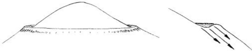
Figure 9.14 A swale is a ditch cut along a contour. Water is held in the ditch until it soaks into the soil.
