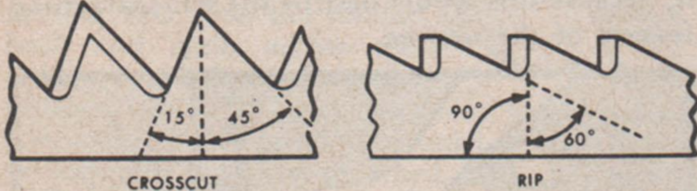
SIDE VIEWS—SHOWING PROPER TOOTH ANGLES
